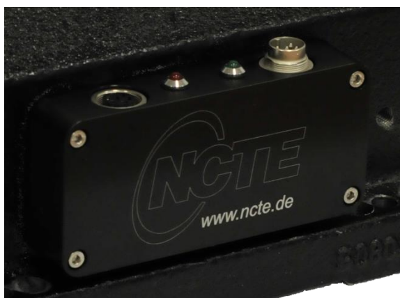
Status LEDs on the electronic box
